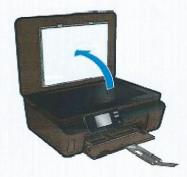
b. Load original print side down on the right front corner of glass.
